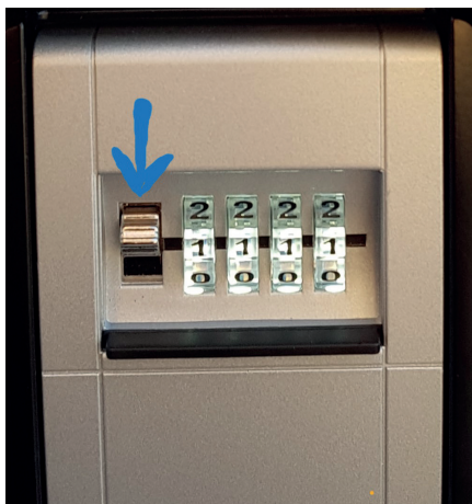
5. Enter the four-digit PIN and press the button down.
